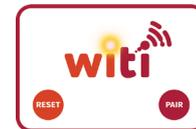
5. While the WiTi Wireless Communication Module is in PAIRING mode, retrieve the WiTi Wireless Brake Controller. Turn the ignition in the tow vehicle on to ensure there is power available at the 12V cigarette lighter socket. Press and hold the emergency Brake override button on the WiTi Wireless Brake Controller. While the Brake override button is still depressed, insert the WiTi Wireless Brake Controller into the vehicle 12V cigarette lighter socket.
